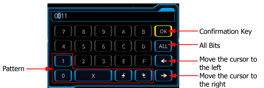
Figure 5-6 Virtual Keypad for Pattern Setting
