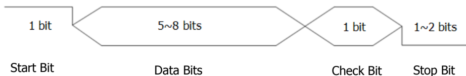
Figure 5-13 Schematic Diagram of RS232 Protocol
