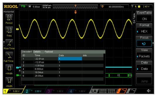
Figure 8-2 Parallel Decoding Event Table
