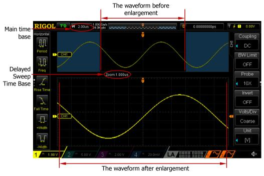
Figure 3-1 Delayed Sweep Mode
