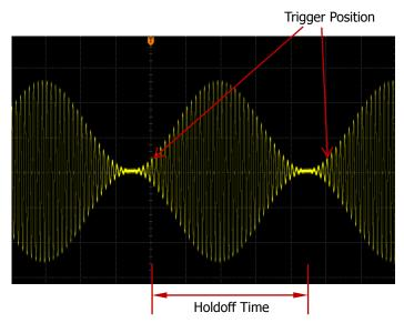
Figure 5-2 Schematic Diagram of Trigger Holdoff
