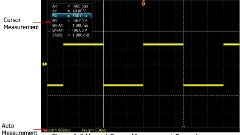
Figure 6-6 Manual Cursor Measurement Example
