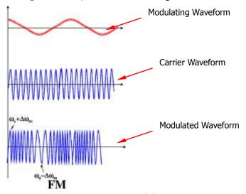
Figure 13-11 Frequency Modulation
