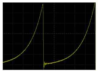
Figure 13-4 Built-in Waveform-ExpRise
