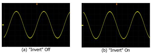
Figure 2-1 Waveform Invert
