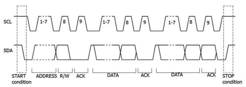
Figure 5-14 Schematic Diagram of I2C Protocol
