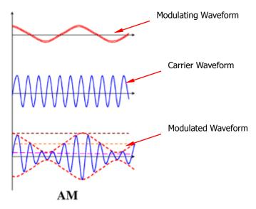
Figure 13-10 Amplitude Modulation
