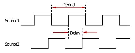
Figure 6-4 Delay and Phase
