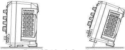
Figure 1-3 To Adjust the Supporting Legs
