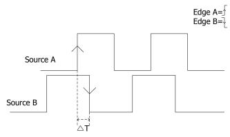
Figure 5-10 Delay Trigger
