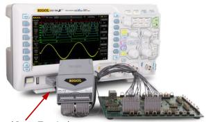
Digital Channel Input Terminal Figure 1-6 To Connect the Logic Probe
