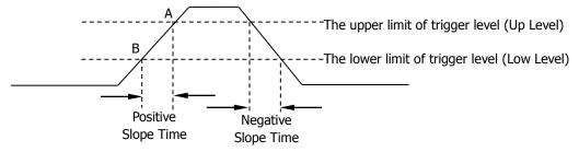
Figure 5-4 Positive Slope Time/Negative Slope Time
