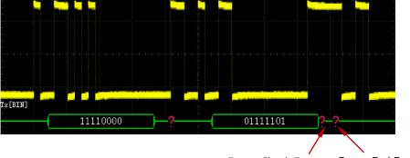
Frame Check Error Frame End Error
