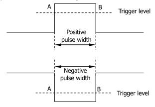
Figure 5-3 Positive Pulse Width/Negative Pulse Width
