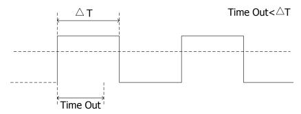
Figure 5-8 TimeOut Trigger
