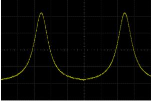
Figure 13-8 Built-in Waveform-Lorentz
