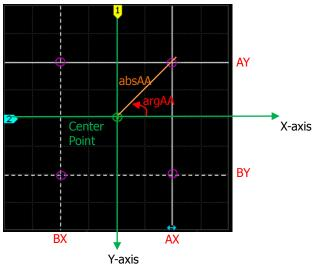
Figure 6-8 XY Cursor Measurement Definition
