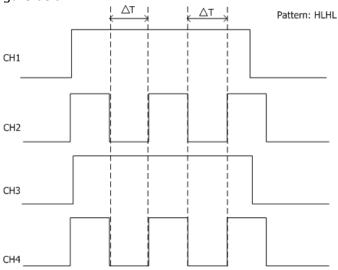
Figure 5-7 Duration Trigger
