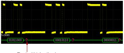
The stop bit is less than 1
