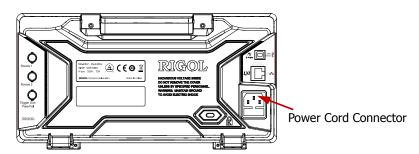
Figure 1-4 To Connect to Power Supply
