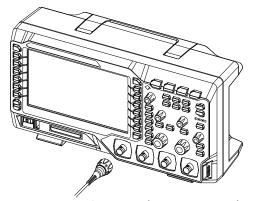
Figure 1-5 To Connect the Passive Probe
