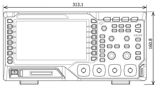
Figure 1-1 Front View Unit: mm
