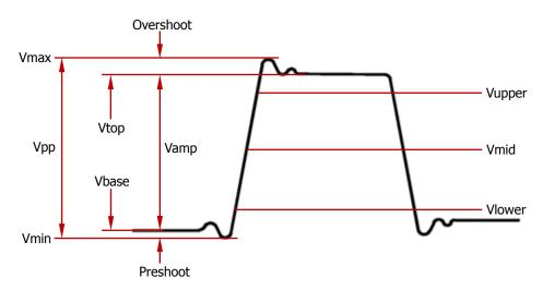
Figure 6-5 Voltage Parameters
