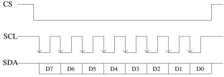
Figure 5-15 Sequential Chart of SPI Bus
