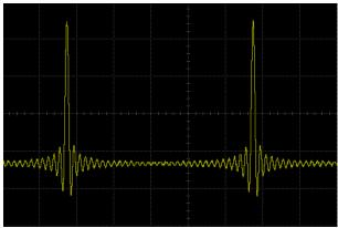
Figure 13-3 Built-in Waveform-Sinc
