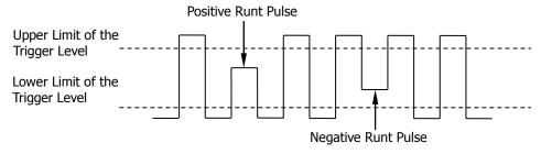
Figure 5-9 Runt Trigger
