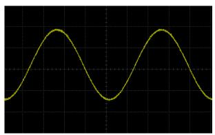
Figure 13-9 Built-in Waveform-Haversine
