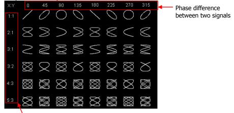
Frequency ratio between two signals
