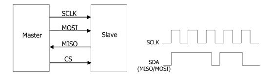
Figure 8-1 SPI Serial Bus
