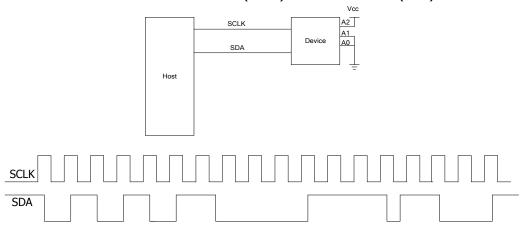
Figure 8-5 I2C Serial Bus
