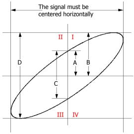
Figure 3-2 Measurement Schematic Diagram of Phase Deviation
