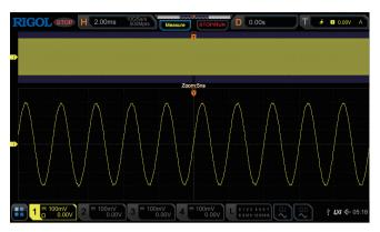
With up to 500 M memory depth, you can capture 50 ms of waveforms while maintaining a sample rate of 10 G, without causing the waveforms to be distorted
