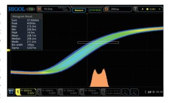
Histogram of Horizontal Waveforms
