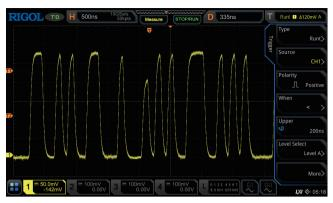
The Runt trigger helps you capture the runt pulse signal in the pulse train
